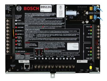
The B9512G Control Panel and the B8512G Control Panel are the new premier commercial control panels from Bosch. B9512G control panels integrate intrusion, fire, and access control providing one simple user interface for all systems. With the ability to adapt to large and small applications, the B9512G provides up to 599 individually identified points that can be split into 32 areas.
